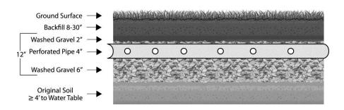
Image 3: Drainfield - Cross Section View
